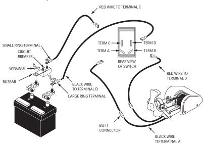
Figure 2. Deckmate 19 Wiring
